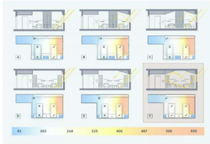
Figure 15. Comparative study of ceiling conformation and furniture arrangement according to natural light distribution. Option (A): Furniture centrally located between the two beds; no suspended ceiling. Requirements are not met. Option (B): Furniture placed centrally between the two beds; suspended ceiling on only one side of the room. Requirements are not all met. Option (C): Furniture placed centrally between the two beds; suspended ceiling on a both sides of the room. Requirements are not all met. Option (D): Furniture placed between each bed and adjacent wall; no suspended ceiling. Requirements are not all met. Option (E): Furniture placed between each bed and adjacent wall; false ceiling on only one side of the room. Requirements are not all met. Option (F): Furniture placed between each bed and adjacent wall; suspended ceiling on a both sides of the room. All requirements are met.
