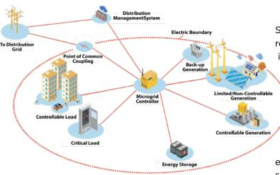
For reliability, security and cost-effectiveness, owners should utilize as much of their existing essential electrical system as possible in a microgrid, including preinstalled onsite switchgear, electrical distribution feeders, backup generators, etc. to reduce implementation costs.
